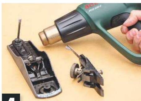
**4** Wash off grey deposit from metal surfaces with abrasive pad. Rinse and dry components with heat gun
